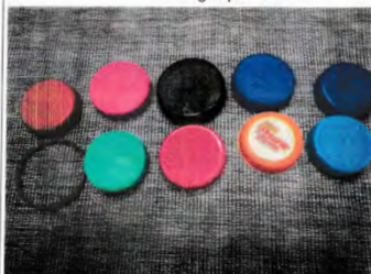
Detergent Caps with white gasket and label removed
