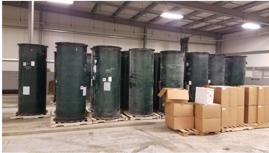
Grinder Pump Basins in Storage
