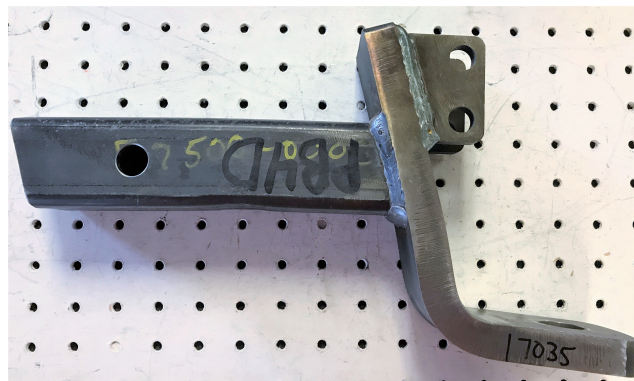
Following Overload – 1.6° Bend in Tube and 5.9° in Ball Platform
