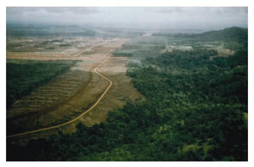
An aerial view of an anti-ambush clearing on each side of a road by Rome plows
