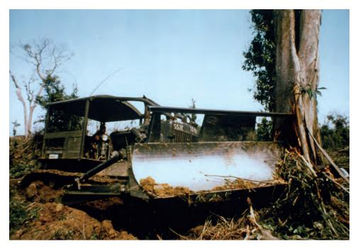
A modified D7E bulldozer equipped with a Rome plow and an armored cab
