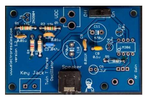
Stage 4 - At this step, add polarized capacitors C5, C6, C7, C10 & C11. Polarity is important, make sure to align the component +/- with the board markings for +/-
