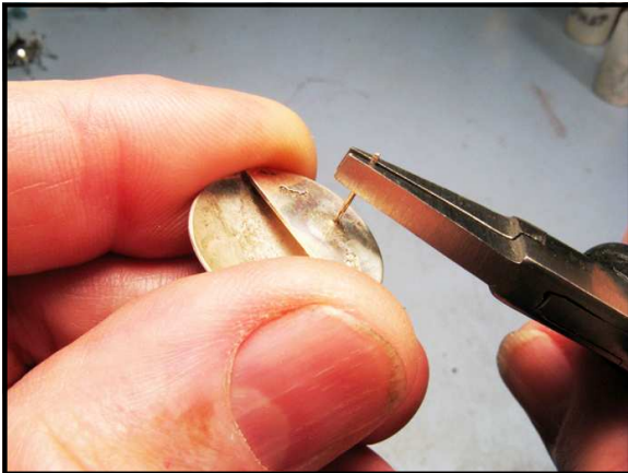
Two half-twists hardens the wire and checks the soldered joint.
