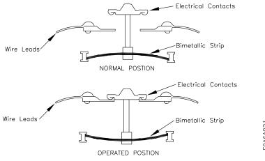
Figure 6-3 Bimetallic Thermostat
