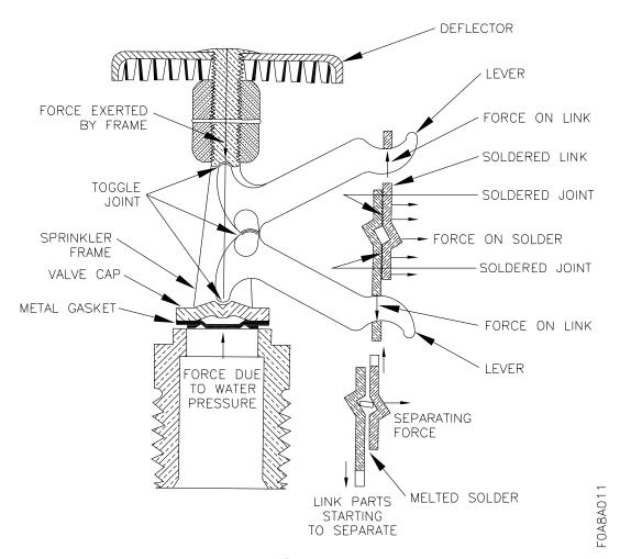
Figure 8-1 Sprinkler Heads
