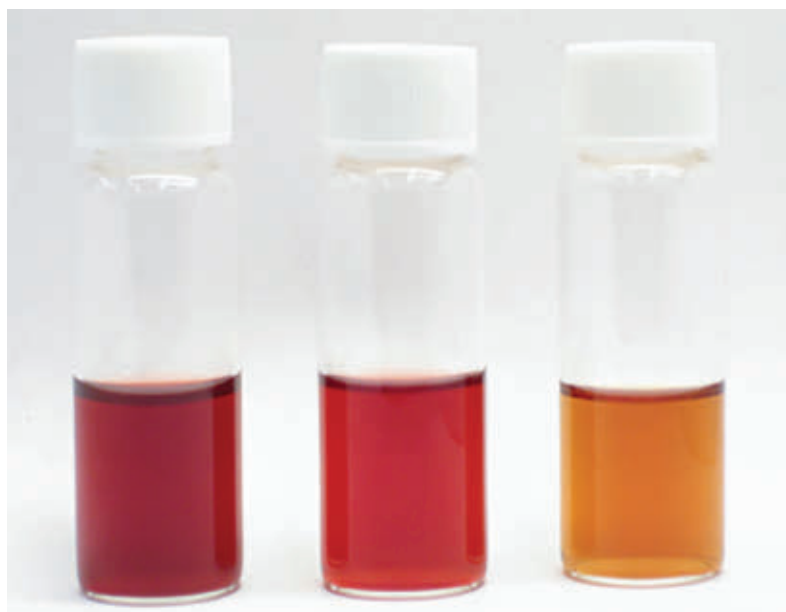
● Figure 2. Three different anthocyanins produced via E. coli (from L): peonidin 3- O -glucoside, cyanidin 3- O -glucoside and pelargonidin 3- O -glucoside
