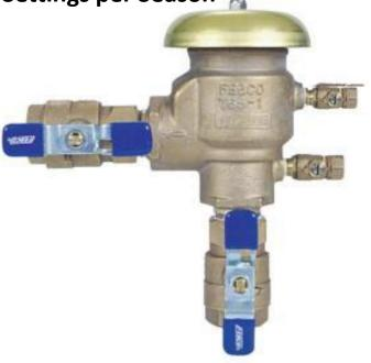
Winter Settings with System Off (all ports cocked at 45 degrees) drain caps open Spring Settings with System On- Ports at 90 degree vertical lines and handles flush with pipes
