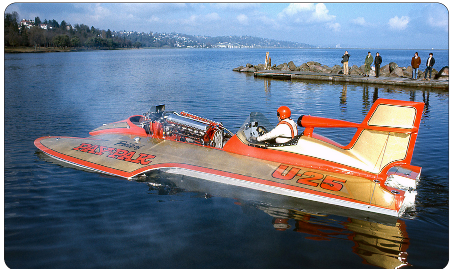
TOP: During the winter of 1970-71, the two Chrysler Hemi engines in Pride of Pay 'n Pak were replaced with a Rolls-Royce Merlin engine and the boat was rebuilt to put the cockpit behind the engine. MIDDLE: David Smith also redesigned the boat's tail. ABOVE: The converted Pride of Pay 'n Pak during its test runs in Seattle before the 1971 season.
