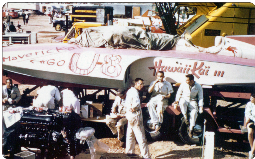
While at Lake Tahoe in 1960, the Hawaii Ka'i crew rebuilt the boat's sponson with some plywood left over from the Maverick . As a nod to the source of the repair, Burns Smith jokingly painted "MavericKai" on the rebuilt sponson.
