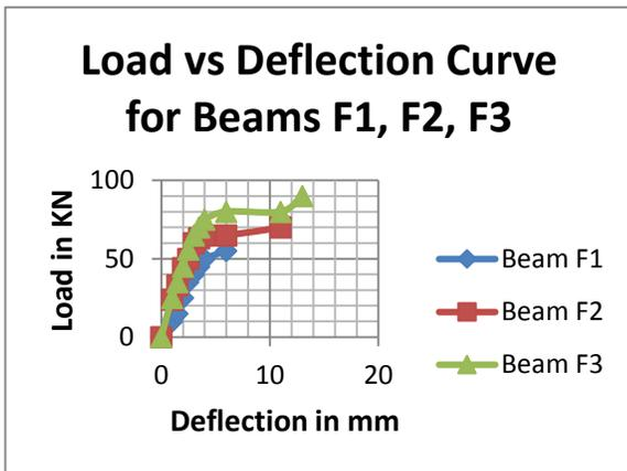
Load vs. Deflection Curve for Beams F1, F2, F3
