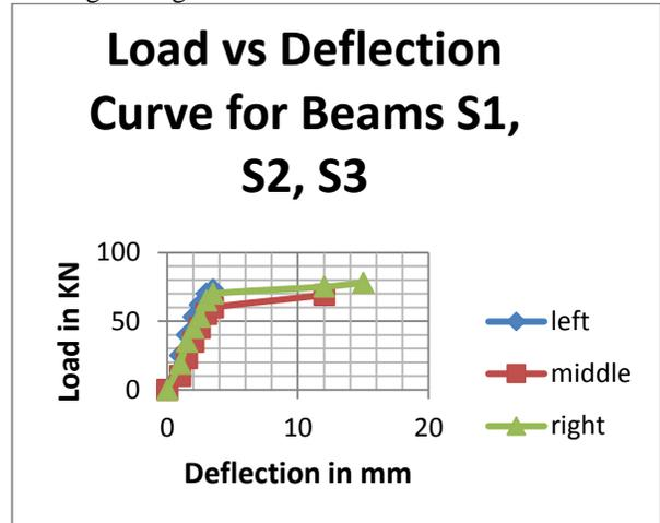
Load vs Deflection Curves for Beam S1, S2, S3
