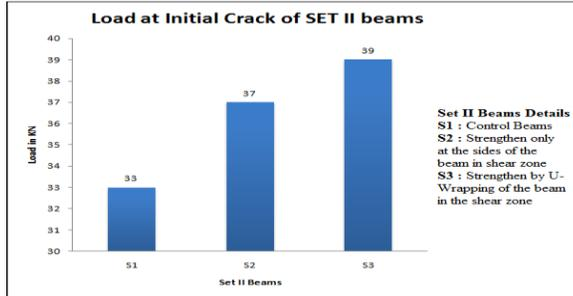
Load at initial crack of beams S1, S2, and S3
