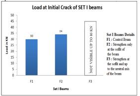
Load at initial crack of beams F1, F2, and F3
