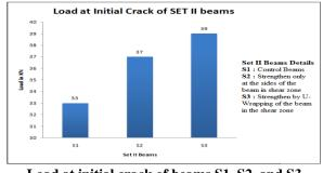
Load at initial crack of beams S1, S2, and S3
