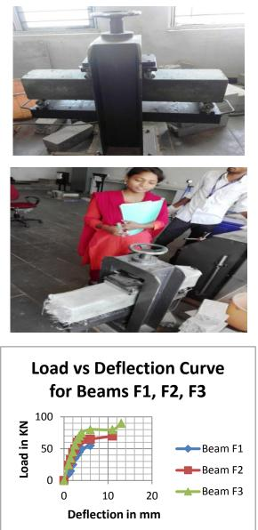
Load vs. Deflection Curve for Beams F1, F2, F3
