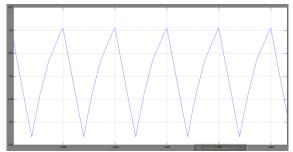
Fig.4: Voltage o/p at load in step down mode
