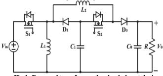
Fig.1: Proposed transformer-less buck-boost device
