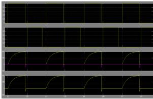
Fig.13 Commutation signals, i/p inductor currents and i/p fuel cell current
