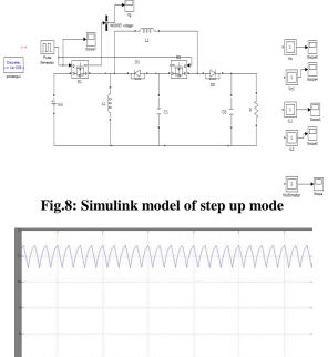
Fig.9: Capacitor (C1) and load resistances voltage graph of step up mode
