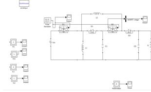
Fig.2: Simulink model of step down mode
