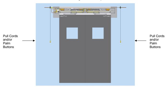
All Regulators & Valves are Self-Contained within Operator Case!
