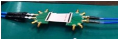
Case2, Connector to Connector Use two test Fixtures
