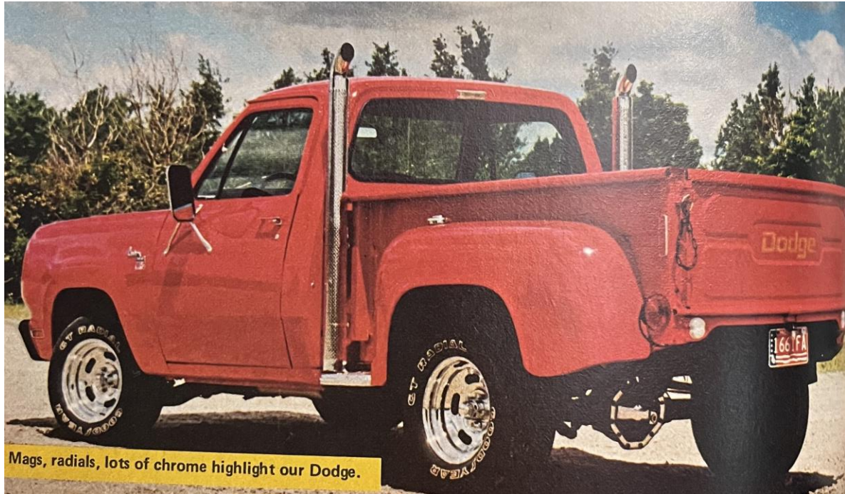
Color pics from "Street Crusin'" magazine, October 1977 (notice "Charger style" fuel filler cap on top of rear fender & side marker lights on rear bed stake pocket, small stainless shields on exhaust.)
