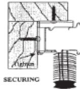
**NOTE:** If more than two brackets are required, insert the headrail in the center brackets first. If necessary, tighten the screws on the center bracket to hold the headrail in position allowing insertion into the other brackets. Tighten screws in bottom of bracket.
