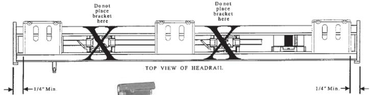
Tab slopes downward giving a lead-in for the insertion of the headrail from the front.
