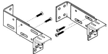
**END MOUNT APPLICATIONS:** End mounting is used when the headrail must span an open space - an arched window opening, for example.
