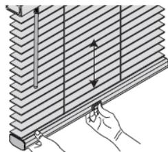
**TO LOWER BLIND:** Prior to lowering the blind, fully press the center button with your thumb and pull the bottom rail down to the desired height while the button is fully depressed. Once the blind reaches the preferred position, hold it there while releasing the button and the blind will stay in that position.
