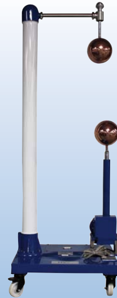
Measuring Spark Gap
