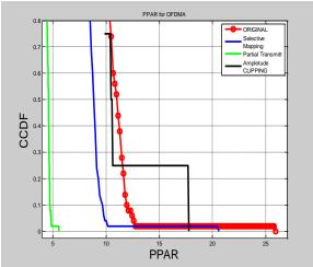
Fig.10: PAPR of OFDMA from different scheme
