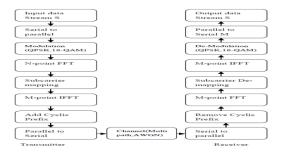
Fig.5: Transmitter Receiver systems for SC-FDMA
