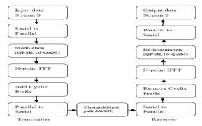
Fig.3: Transmitter Receiver system for OFDM
