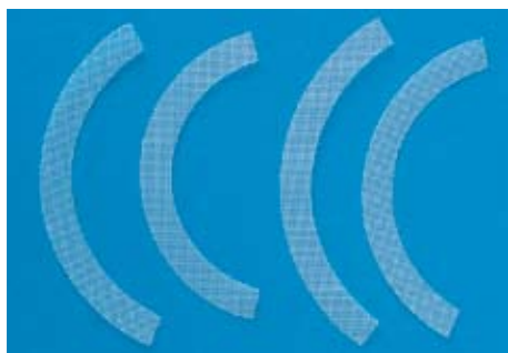
Fig. 1: Four different curvature shapes Two B-shapes, more curved Two A-shapes, less curved Both available in nylon fiber, .25 mm thick and stainless steel, 0.02 mm thick
