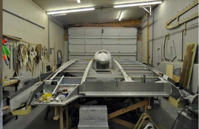
including deck work. The new hull is in the basic framework configuration with no hardware, components, or systems in the boat at this stage.
