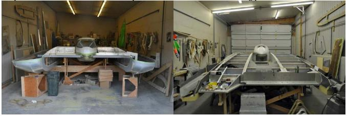
including deck work. The new hull is in the basic framework configuration with no hardware, components, or systems in the boat at this stage.
