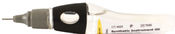
12 ml Synthetic Oil Pen T030 To avoid fretting corrosion Apply a drop of lubricant after cleaning and before sterilization on all joints, threads, and sliding surfaces
