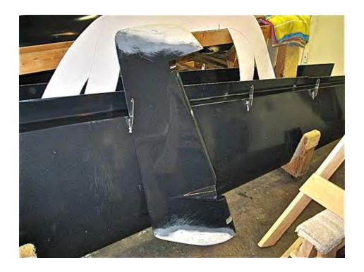
Not one to complain, but I was not happy with the rudder support stop bushings on the rudder support tube. So .... again I made my own. An option for this would be for the kit to include two more bushings in the kit. Shown is how they turned out in my case.
