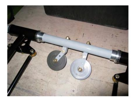
Finally, there a picture of how I centered the bolt holes on the 1/2" bar stock for the universal joints. Actually, I used a model airplane centering jig used for slotting the hinges on balsa wood to center the holes.
