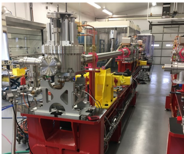
FIGURE 7. Front end undergoing leak testing; viewed from the downstream end.
