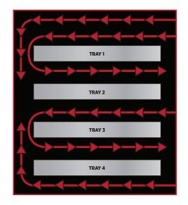
HVHA Sterilization moves heated air rapidly and provides shorter start-to-finish pre-set cycles as well as faster, more effective sterility.
