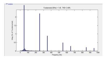
Fig. 7 shows using SAPF the source current harmonics are reduced with low THD that means 2.44%.
