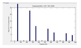
Fig. 6 shows Before compensation with nonlinear load the source current harmonics are high, and THD was 30%.
