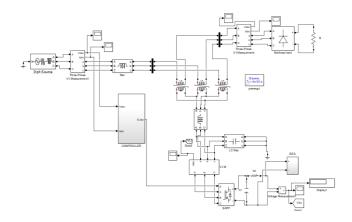
Fig 5 MATLAB simulated schematic diagram of proposed system
