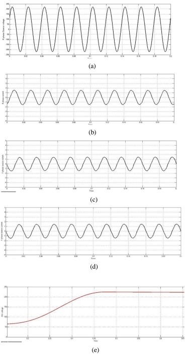
Fig. 5 SAPF response of nonlinear system (a). R phase grid voltage, (b). R phase grid current, (c). Y phase grid current, (d). B phase grid current, (e) DC link voltage
