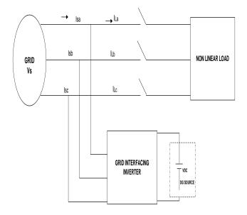
Fig. 2 Grid connected DG interface
