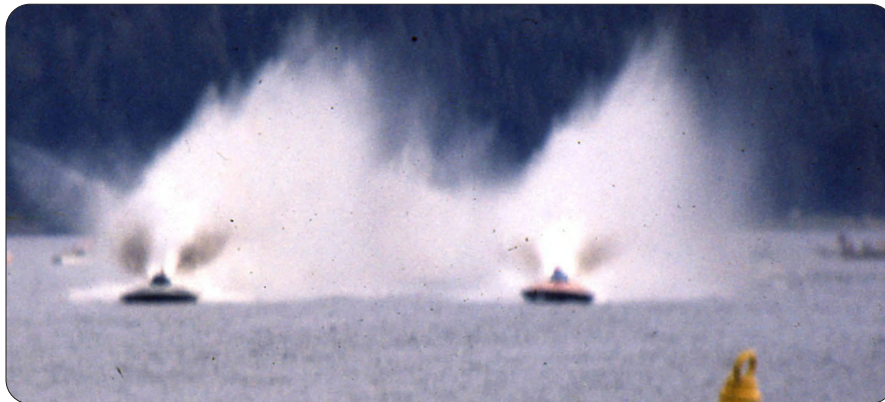
Black smoke erupted from the exhaust stacks of both Miss Bardahl and Miss Exide when their drivers gave the engines a shot of nitrous oxide for quick acceleration.
