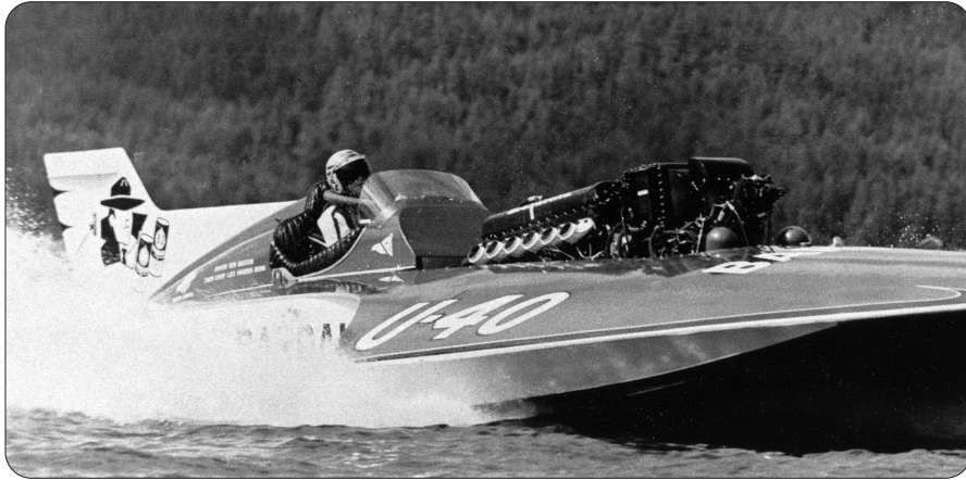
The top of the two nitrous oxide bottles can be seen in front of the engine.
