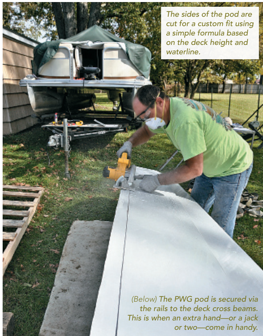
Aluminum Performance Sheeting panels are installed under the deck to deflect and direct water flow around the PWG pod.
