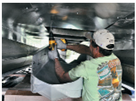
Aluminum Performance Sheeting panels are installed under the deck to deflect and direct water flow around the PWG pod.
