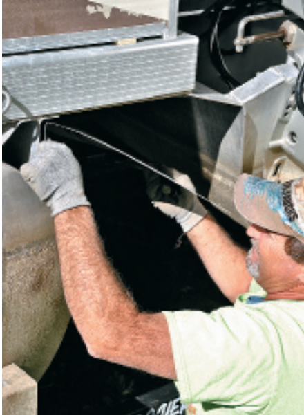
Aluminum Performance Sheeting panels are installed under the deck to deflect and direct water flow around the PWG pod.
