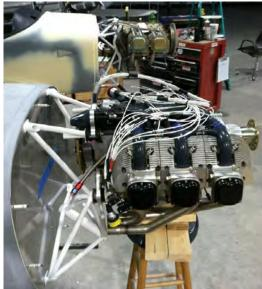
Left photo, Doug and Ronda Guy install their UL Power 390iS. They will be the first Lightning in the US to fly with this engine. On the right is their engine in the foreground with a Superior O-320 in the background. Both are 160 HP.
