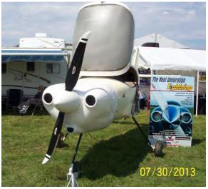
More photos of the new 160 HP Lightning. Note the longer gear legs which allow for a longer prop with good ground clearance. Photos by Dale Fowler.
