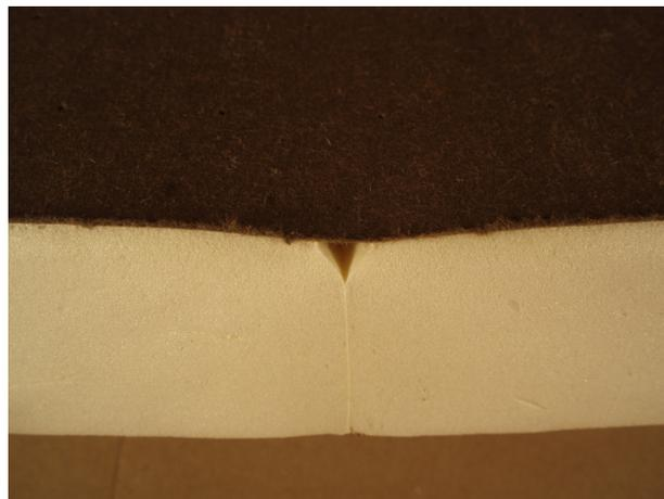
Knit line and V-groove close-up (after conditioning)
