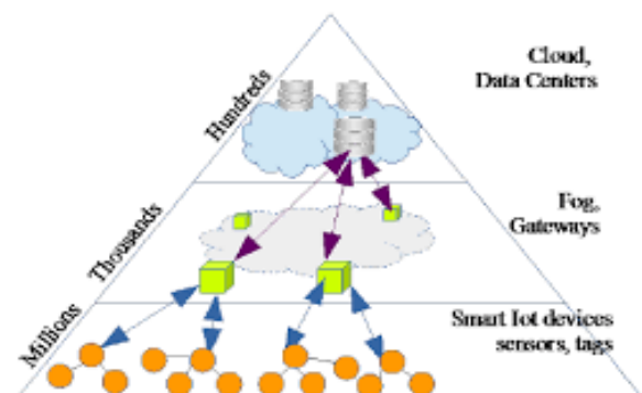
Fig.4: Fog computing works as a bridge between Cloud and end devices
