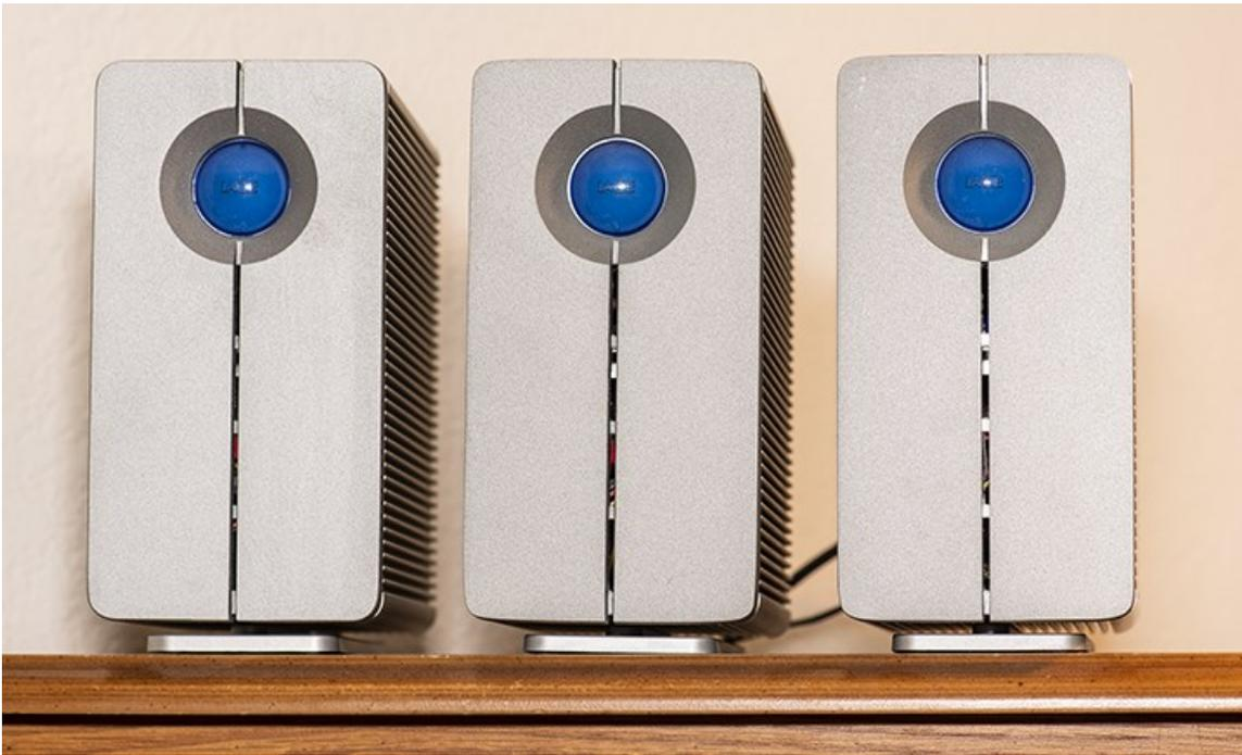
*The three units pictured above are a RAID system. Each box contains two independent drives, with an electronic controller. It provides a seamless, user-friendly method of safely backing up the images through redundancy. The process is managed by the internal RAID controller. Each unit is a 20TB RAID. When used together, the system will store 60TB of data, providing 30TB of file storage with an equal amount of redundant backup.*
