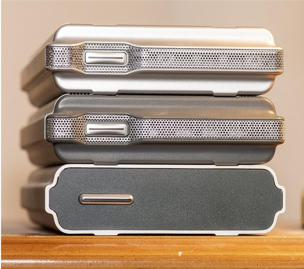
*Some manufacturers offer drive systems that enable expansion as required. The three drives above are tied together in JBOD system. But, management of file storage and redundancy is a continuing issue.*
