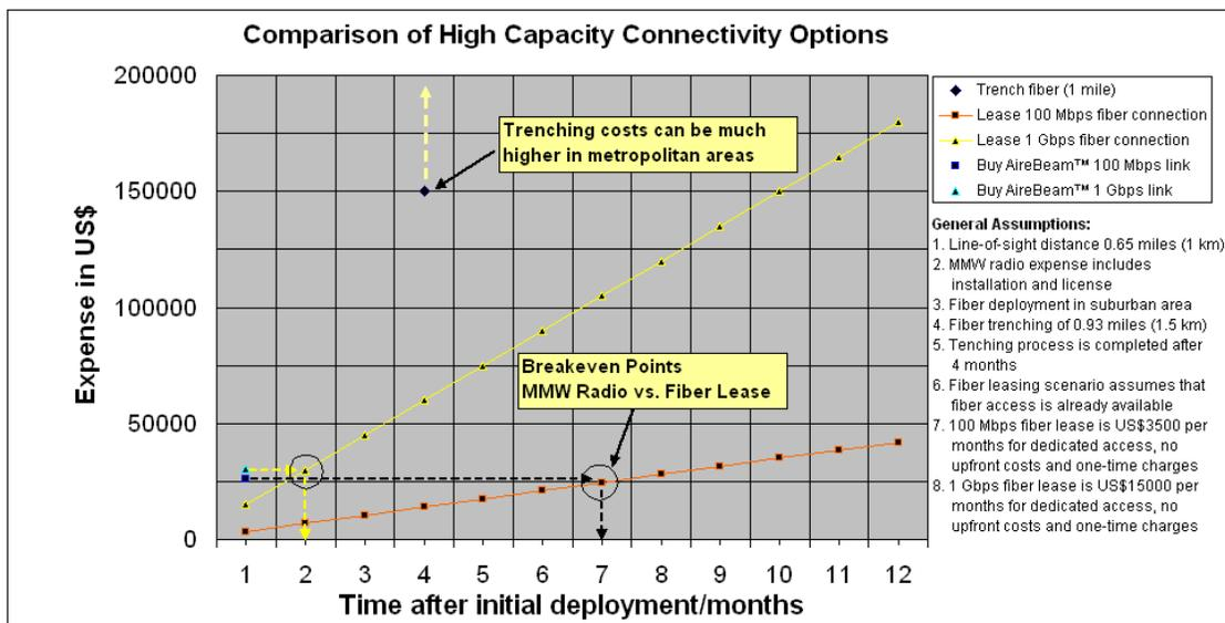
**Figure 3:** A financial comparison of different high capacity “Last Mile” access strategies: Trenching fiber, leasing a fiber connection, using a MMW radio solution.
