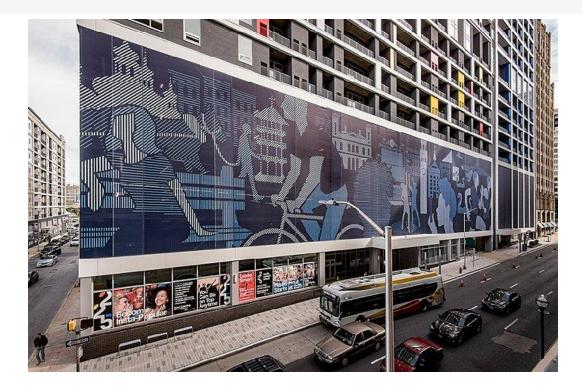
This building wrap includes 22 panels, most are 20'w x 45' high. The corner is one graphic panel wrapped on both facades, the multi-frame junctions create a seamless graphic that wraps the majority of a city block.
