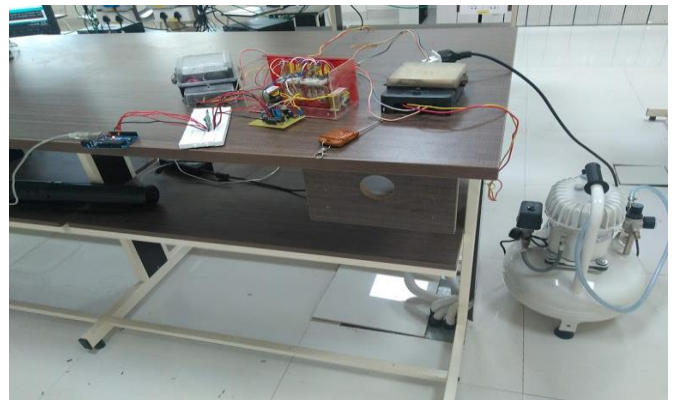
Figure 11. Air Compressor as electrical load
