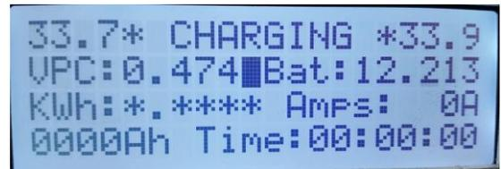
2) **BAT:** The battery nominal voltage is set to match the battery voltage you are working with. The battery voltage must be set correctly, or the machine may not function.
