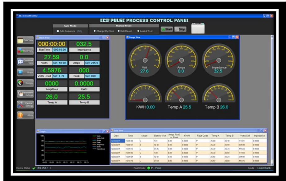
BZI has developed a PC based, Graphical User Interface (GUI) shown to the right, that allows the operator to remotely monitor and operate the Model 6000.
