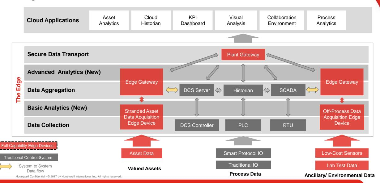
New EDGE devices developed to meet data collection, transport and analytics needs.
