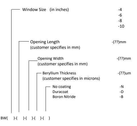
For example: to order a 10 Inch Beryllium window, with an opening length of 10mm, an opening width of 40mm with a beryllium thickness of 250 microns, and a baron nitride coating, the part number would be:
