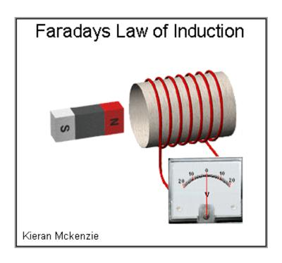
Any change in the magnetic environment of a coil of wire will cause a voltage to be "induced" in the coil.
