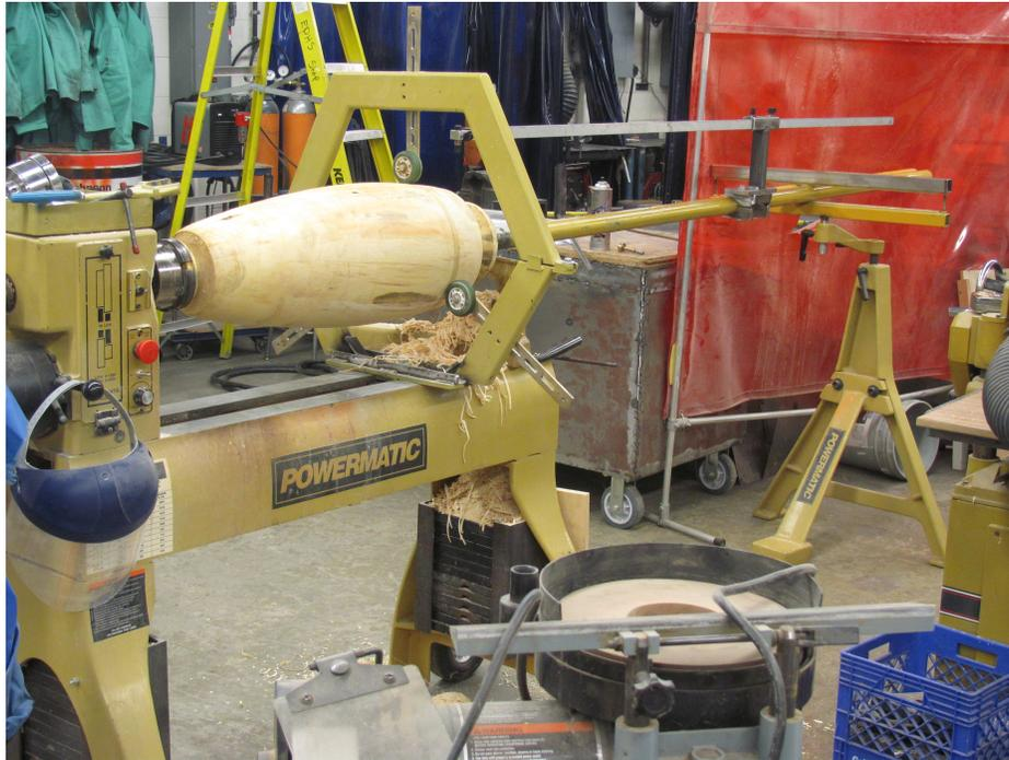
First, this article covers hollowing to depths that commercial boring bars will not go, in excess of thirty inches (76.2 CM) deep. The deeper/bigger you go, the difficulty/danger expands exponentially. **Also, DO NOT forget how dangerous it is to have several hundred pounds of rotating mass in your lathe, which can turn lethal in a heartbeat!**
