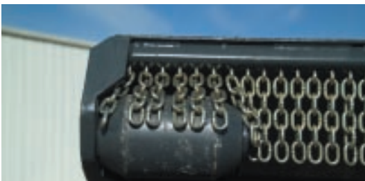
Front rollers allow attachment to better traverse uneven terrain while reducing operator fatigue. Standard equipment on all Brushcat rotary cutters.
