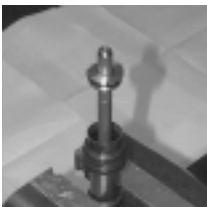
Install rebound seal head
