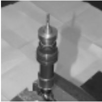
Insert pressure piston
