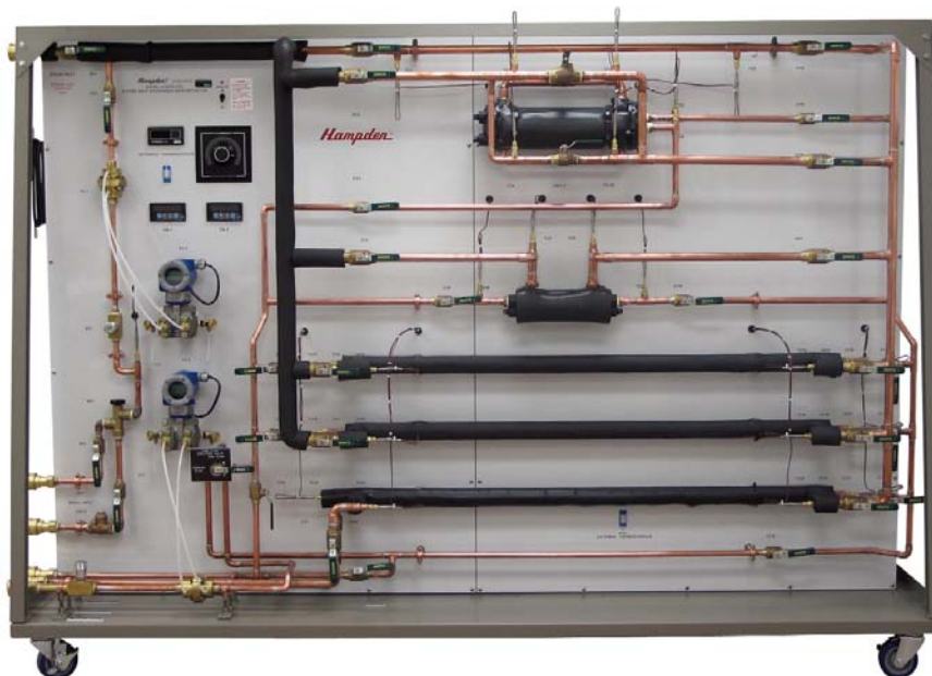
Model H-6878-CDL 6-Pass Heat Exchanger Demonstrator with Computer Data Logging option. Dimensions: 78"H x 94"W x 31"D, Weight: 600 lbs.
