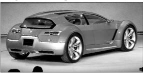
The Dodge ZEO Concept (above) is an allelectric "2+2" sport wagon with rear wheel drive, what looks like the same 200 kW motor as the other two, but a 64 kWh li-ion battery that gives 250 mile range. With a curb weight of 3400 lbs it hits 60 in 5.7 s, does the quarter in 11 s even, and hits 130 mph.
