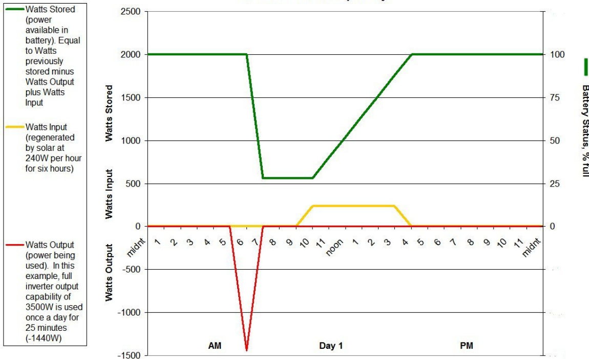
Sustainable Max Inverter Output Example 3500 W/hr for 25 minutes once a day Six hours sunshine per day
