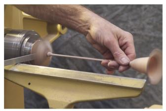
21 Extra credit: you can remove the tail stock and support the spinning stem with your hand and then part the goblet completely off.
