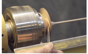
19 Start making slow parting cuts at an angle into the bottom of the base being careful not to catch the top edge of the parting tool on the rim of the base as it starts to get thin.
