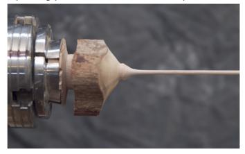
18 As you near the bottom section where you left the bark, form the base and add any detail you like at the base of the stem. Sand the base.
