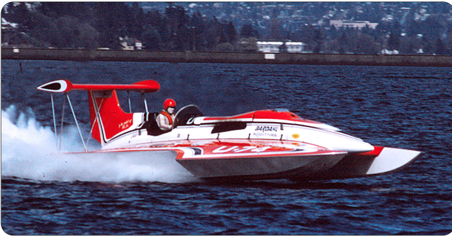
TOP: Ron Jones introduced the sport to the horizontal stabilizer, or wing, with the creation of the "Winged Wonder" Pay 'n Pak in 1973. ABOVE: Pay 'n Pak was so successful, other boat owners soon ordered hydros from Jones that also sported wings. An example is Weisfield's , which was built in 1974.
