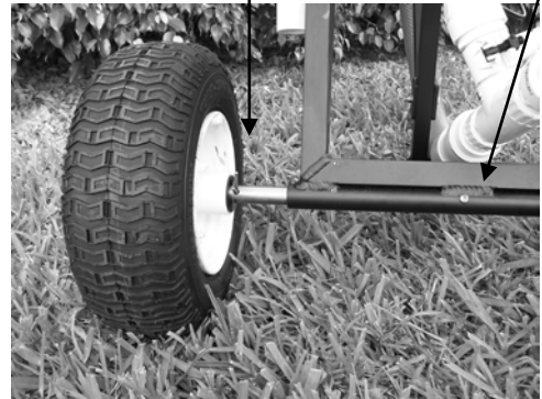
(Picture 8) Insert axle and tighten nylock nut. Slide wheel and tire assemblies onto axle and pin Seq. of assembly- Pin, washer, wheel, washer, pin.
