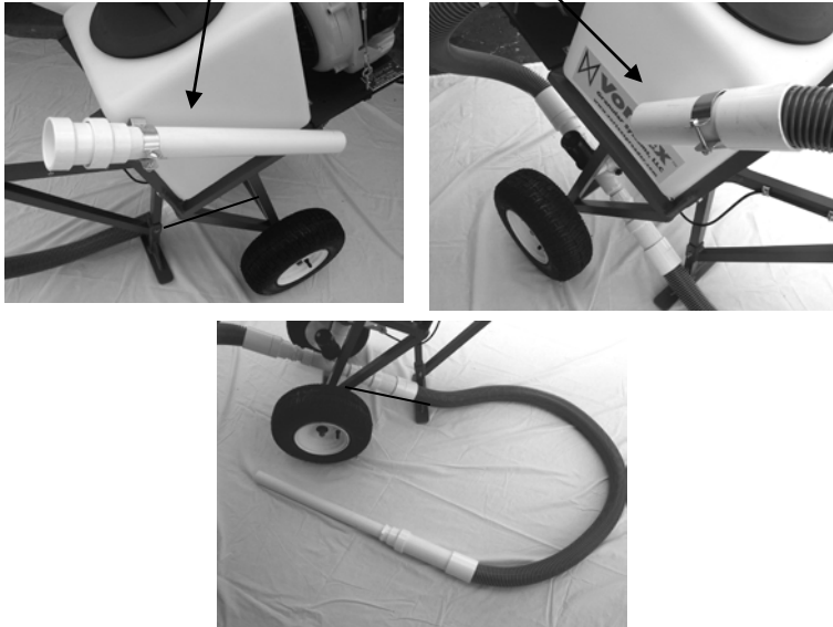
(Picture 9) Place extension tubes and fertilizer hose in holders
