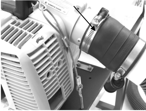
(Picture 7) Attach quick clamp to blower hose
