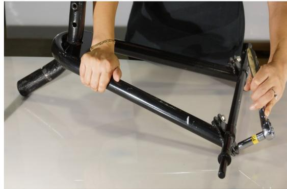
**Step 2**—Bolt axle to the main lower main frame.
