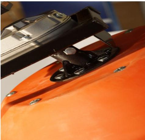
**Step 16**— Install the large bolt and tighten the Lock nut.
