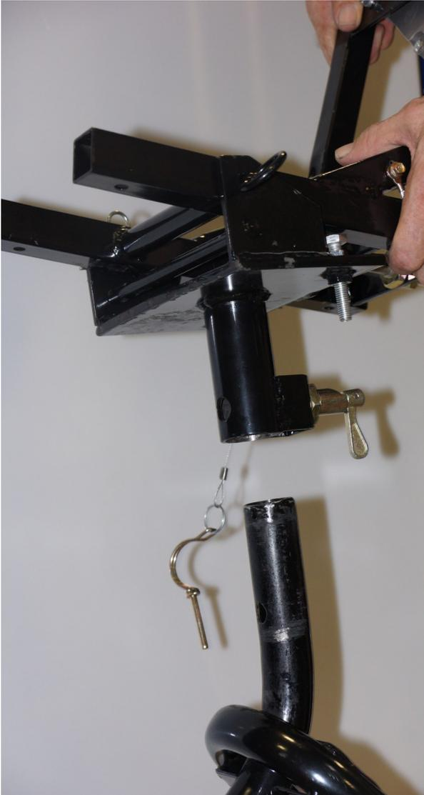
**Step 13** – Lift the tilting main frame and slide over the lower main frame pull back the swivel latch first.
