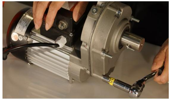
**Step 6** -Tighten the inner nuts to about 10 pounds torque.
