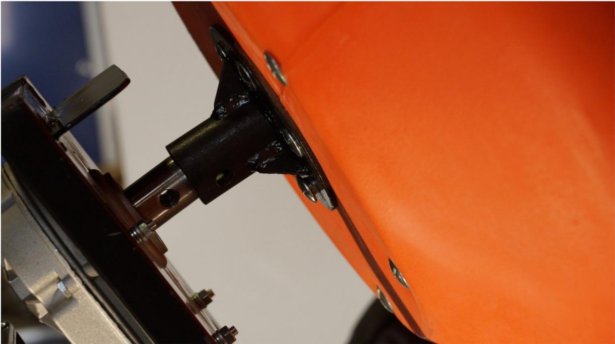
**Step 15**— Slide the drum on to the shaft of the gear motor. Turn so the hole lines up.
