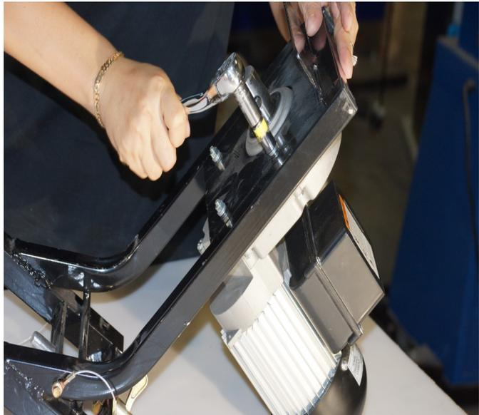
**Step 10** — Install flat washer, spring washer and nut and tighten to 10 lbs torque.
