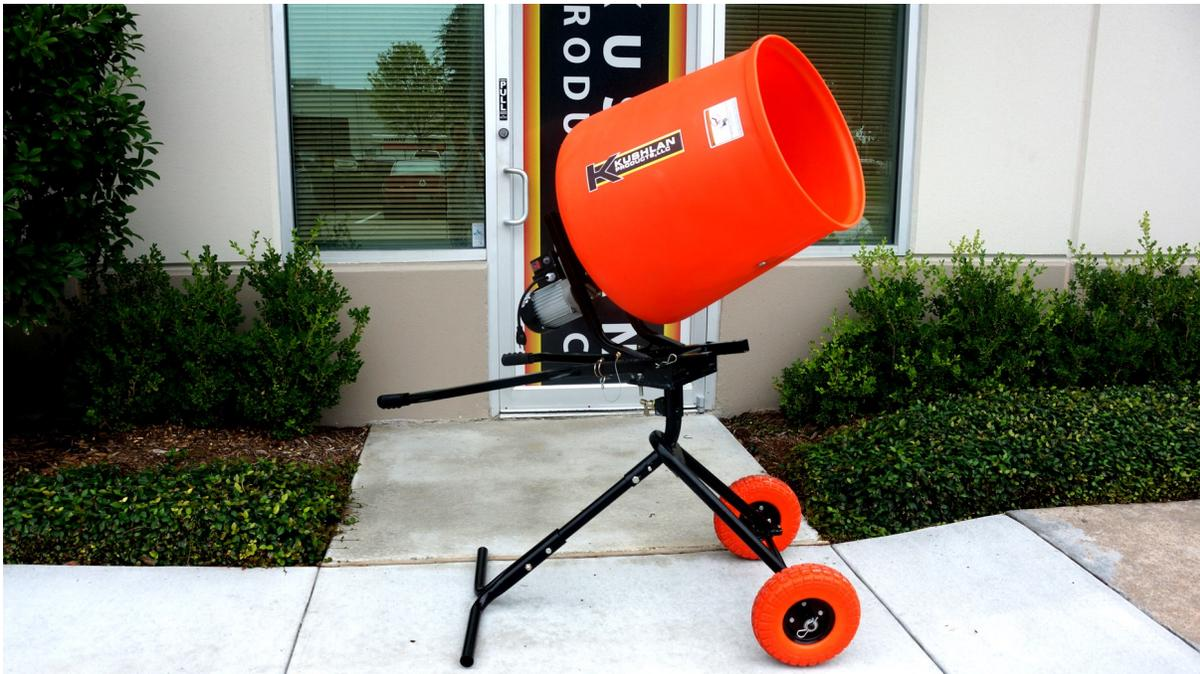
**Step 19** - Rotate to 180° to the lock out position dump raise the handles and dump the concrete out onto either a wheelbarrow or directly onto the work you are doing. By pulling the swivel latch and rotating at 180° to the lock out position, the mixer will rotate 360°.
