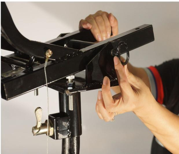
**Step 11**— Tilting the mainframe by installing the large pivot pin.
